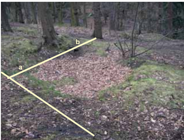
Plan survey showing base and transect lines.
